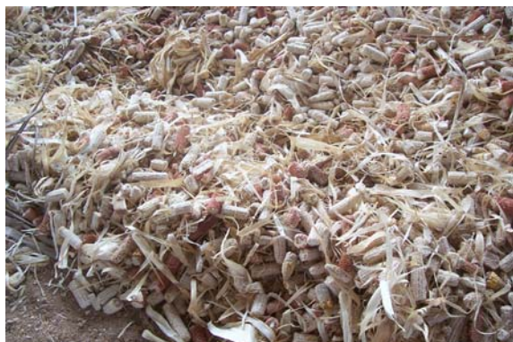
Photo 15: Corn cobs cause fouling in furnace. Furnace must have water wall without refractory.
