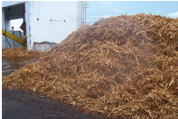
Photo 13: oversized wood chips – cause interruption in fuel feeding
